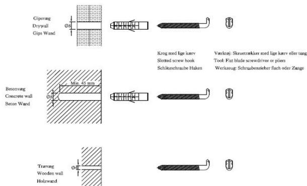
Template for drilling for mounting screws.
