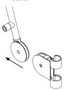
14. Slide the bracket and arm onto the pole.
